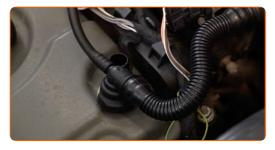
Remove the crankcase ventilation hoses.
