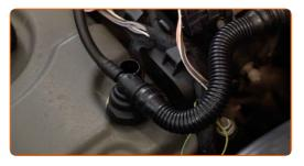
Remove the crankcase ventilation hoses.
