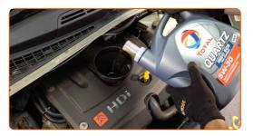
Replacement: engine oil and filter – CITROËN Xantia Box Body / Estate (X2). Tip:
