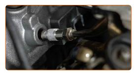
Tighten the glow plugs. Use the spark plug socket #12. Use a torque wrench. Tighten it to 25 nm torque.
