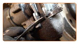
Remove the brake pads. Use a crowbar.
