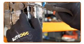
Remove the brake pad retaining pin. Use round-nose pliers.
