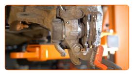
Remove the retainer of the brake pads. Use a crowbar. Use a rubber mallet.
