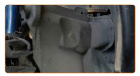
Install and tighten the wheel arch cover fasteners. Use a clip removal tool. Use a Phillips screwdriver.
