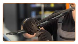
Remove the blade from the wiper arm.
