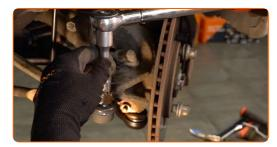
Tighten the tie rod end locknut. Use a combination spanner #19 (2 pieces). Use a torque wrench. Tighten it to 62 nm torque.
