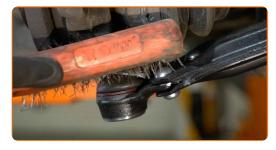
Unscrew the lower fastener connecting the shock strut to the steering knuckle. Use a combination spanner #16. Use a drive socket #16. Use a ratchet wrench.
