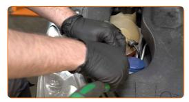
Remove the coolant reservoir cap.
