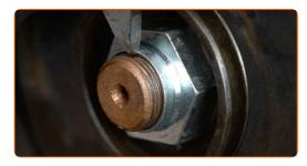
Treat the fastener that connects the suspension strut to the steering knuckle. Treat the ball joint fastener. Treat the fastener connecting the tie rod end to the steering knuckle. Use copper grease.
