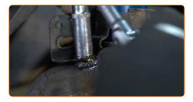
Remove the brake hose bracket.
