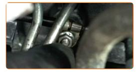
Tighten the fasteners that connect the power cables to the glow plugs. Use a drive socket #8. Use a torque wrench. Tighten it to 8 nm torque.
