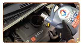
Replacement: engine oil and filter – CITROËN Jumpy Platform / Chassis (V\_). Tip:
