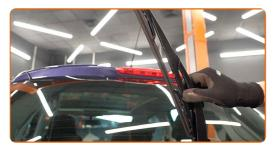
Press the clip. Remove the blade from the wiper arm.
