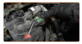
Squeeze the clips and detach the fuel supply lines from the fuel filter housing. Use a flat screwdriver. Use a clip removal tool.
