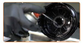
16 Install the new sealing ring.
