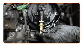
Attach the fuel pressure sensor connector.
