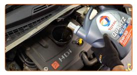
Replacement: engine oil and filter – CITROËN JUMPER Platform/Chassis (244). Tip:
