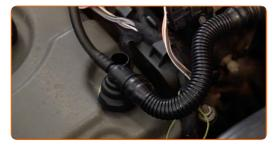
Remove the crankcase ventilation hoses.
