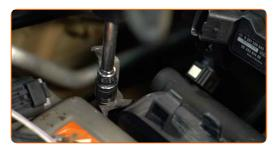
Attach the connector to the intake manifold.
