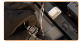
Detach the connector from the intake manifold.
