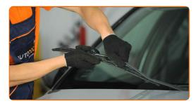
Remove the blade from the wiper arm.
