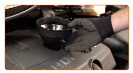
Pour new oil into the engine in the amount recommended by the car manufacturer.
