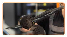
Remove the blade from the wiper arm.
