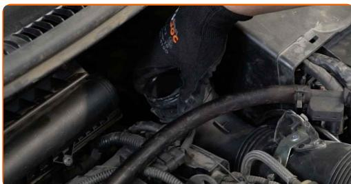
**4** Remove the air intake pipe.
