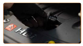
Unscrew the oil filter. Use the 74/76-15F socket.
