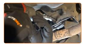
Screw in the engine mount fastener that connects it to the gearbox housing. Use a drive socket #16. Use a ratchet wrench.
