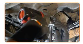
Tighten the fasteners that connect the engine mount to the car body. Use a drive socket #16. Use a torque wrench. Tighten it to 60 nm torque.
