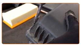
Reinstall the air filter housing.
