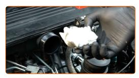
23 Install the air duct.
