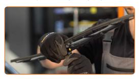
Remove the blade from the wiper arm.
