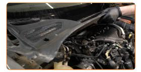
120 Install the fasteners of the wiper plastic cowl grille.
