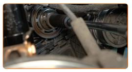
Turn the crankshaft gear. Use a drive socket #22. Use a ratchet wrench.
