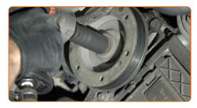
Remove the fastening bolt.
