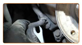
Unscrew the fasteners of the upper timing cover. Use a combination spanner #10.
