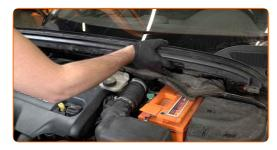
Release the coolant reservoir retainers. Use a clip removal tool.
