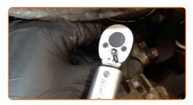
93 Install the crankshaft position sensor.
