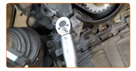
Install the crankshaft gear locking tool.
