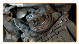
Loosen the fastener of the timing belt tensioner pulley. Use a combination spanner #13. Use HEX No.H6.
