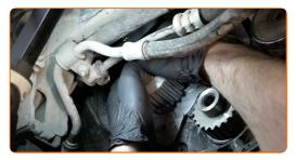
Screw in the water pump fasteners. Use a drive socket #11. Use a ratchet wrench.
