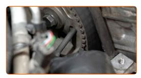
Unscrew the crankshaft pulley fastener. Use a drive socket #22. Use a ratchet wrench.
