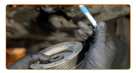
Tighten the crankshaft pulley fastener. Use a drive socket #22. Use a torque wrench. Tighten it to 80 Nm torque.+60°
