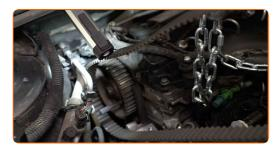
Unscrew the fastener of the timing belt idler pulley. Use a combination spanner #15.
