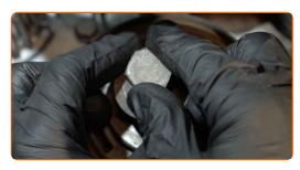
Remove the crankshaft locking tool.
