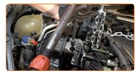
115 Remove the engine support beam.
