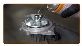
67 Install the water pump gasket.
