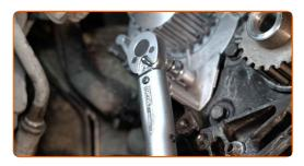
72 Install the timing belt idler pulley.
