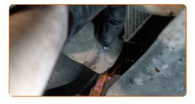
Drain the coolant from the engine.
