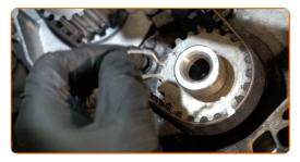
Install the crankshaft gear locking tool.
