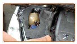
Attach the coolant reservoir using its retainers.
