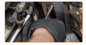
Screw in the crankshaft pulley fastener. Use a drive socket #22. Use a ratchet wrench.
