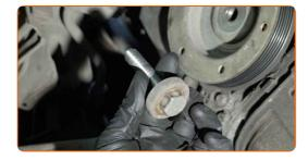
Remove the crankshaft pulley.
