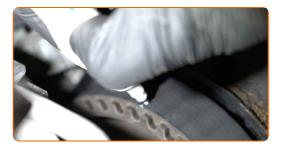
Make a mark on the camshaft gear.
