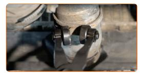
Clean the water pump fasteners. Use all-purpose cleaning spray.
