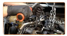
Tighten the engine mount fastening bolts. Use Torx T50. Use a torque wrench. Tighten it to 60 nm torque.
