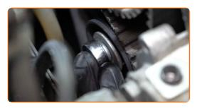
Remove the timing belt tensioner pulley.
