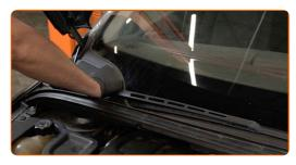
Remove the clips of the plastic cowl grille. Use a clip removal tool.
