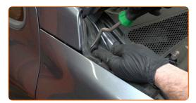
Unscrew the fasteners of the brake fluid reservoir. Use Torx T20. Use a ratchet wrench.
