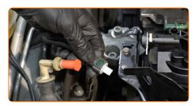
Connect the fuel lines to the fuel filter and lock the fastening clips.
