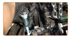
Remove the crankshaft gear locking tool.
