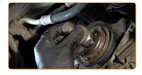
Remove the crankshaft gear locking tool.
