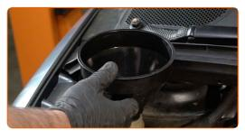
Pour coolant in the coolant reservoir.
