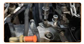
Screw in the fasteners that connect the engine mount to the car body. Use a drive socket #E14. Use a ratchet wrench.
