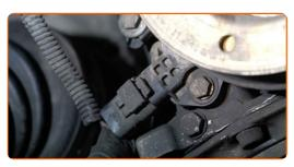
103 Attach the crankshaft position sensor wiring.
