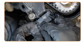
Tighten the fastener of the crankshaft position sensor. Use a drive socket #10. Use a torque wrench. Tighten it to 14 Nm torque.
