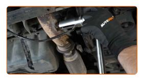
6 Remove the oxygen sensor.
