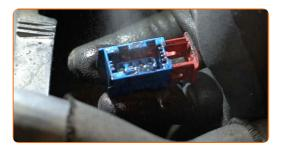
13 Attach the oxygen sensor connector.
