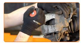
Remove the brake caliper.
