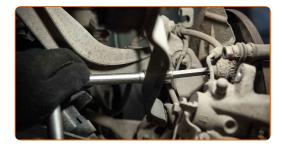
Remove the caliper bracket.
