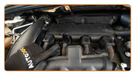
Detach the connector from the ignition coil.
