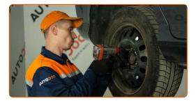
Lower the car and working in a cross order, tighten the wheel bolts. Use wheel impact socket #19. Use a torque wrench. Tighten it to 100 nm torque.
