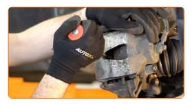
Remove the brake caliper.
