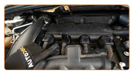
Detach the connector from the ignition coil.
