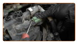
Squeeze the clips and detach the fuel supply lines from the fuel filter housing. Use a flat screwdriver. Use a clip removal tool.
