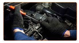
Undo the fastening screws of the air filter cover. Use a Phillips screwdriver.
