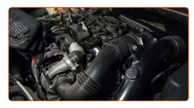
Screw the fastening clamp connecting the air duct to the air filter housing. Use a flat screwdriver.
