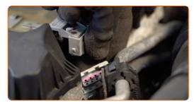
Unscrew the ignition coil bracket. Use Torx T27.
