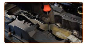
Install the crankcase ventilation hoses.
