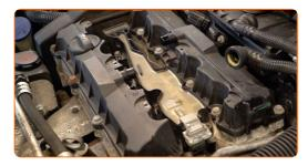
Tighten the fasteners of the ignition coils. Use Torx T20. Use a torque wrench. Tighten it to 8 nm torque.
