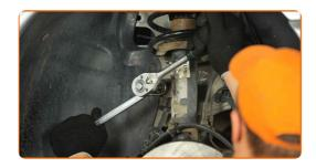
Unscrew the fastener connecting the stabilizer link to the stabilizer bar. Use a combination spanner #18. Use HEX No.H6. Use a ratchet wrench.
