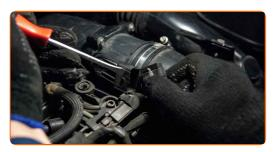
Fasten the clamp on the air intake hose. Use a flat screwdriver.
