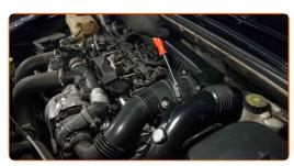
Remove the air distribution housing assembly. Use a flat screwdriver.
