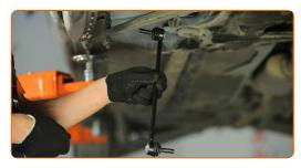
Tighten the fastener connecting the stabilizer link to the stabilizer bar. Use a combination spanner #19. Use HEX No.H6. Use a torque wrench. Tighten it to 65 Nm torque.
