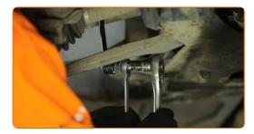
Tighten the fastener connecting the stabilizer link to the shock strut. Use a combination spanner #19. Use HEX No.H6. Use a torque wrench. Tighten it to 65 Nm torque.
