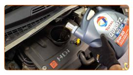
Replacement: engine oil and filter – CITROËN C4 Spacetourer Box Body / Estate (3D\_). Tip:
