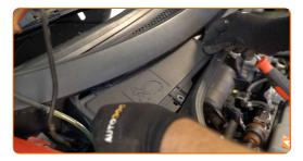
Screw in the fasteners of the cabin filter housing cover. Use a Phillips screwdriver.
