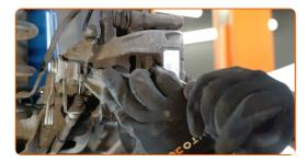
Remove the brake caliper.
