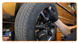
Clean the brake caliper fasteners. Use a wire brush. Use all-purpose cleaning spray.
