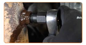
Treat the oxygen sensor. Use copper grease.
