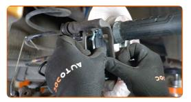
Replacement: brake pads – CITROËN C4 II Box Body / Hatchback (NC\_).
