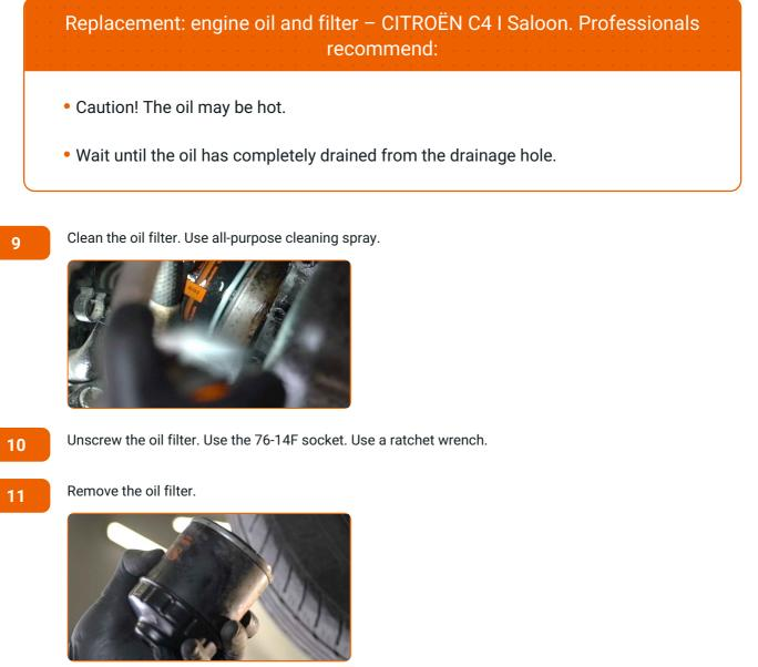
Clean the oil filter seat. Use all-purpose cleaning spray.
