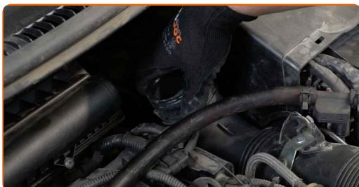
**4** Remove the air intake pipe.
