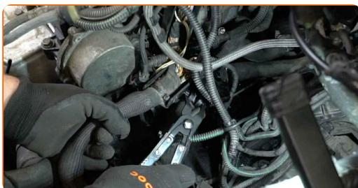
Replacement: engine thermostat – CITROËN C4 I (LC\_). Tip:
