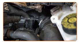
16 Install the brake fluid reservoir.
