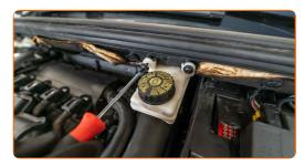
Remove the brake fluid reservoir. Move it aside.
