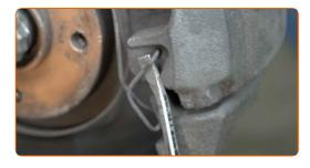
13 Remove the brake caliper.
