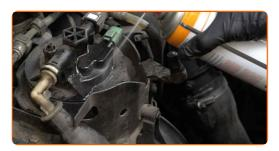
Detach the fuel pressure sensor connector. Use a flat screwdriver.
